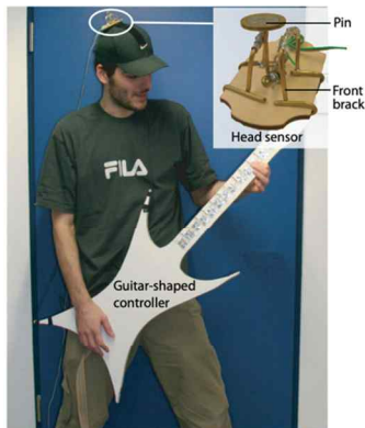
Figure 2. Bardos's Bangarama concept. In this interface, users wear a sensor on their head that will play music when the user "headbangs".
