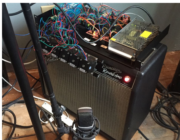
Figure 7. RackFX device-side robotic integration using Arduino controlled stepper motors on a Fender Princeton Reverb guitar amplifier.
